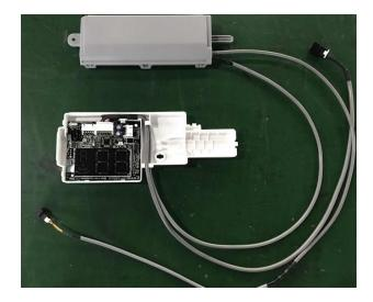
◆ 2-wired cable which could connect to main control PCB board
