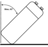
ATTENTION: DUE TO THE HIGH CENTER OF GRAVITY, LOW OVERTURNING MOMENT, THE UNIT MUST BE SECURED AGAINST TIPPING OVER.
