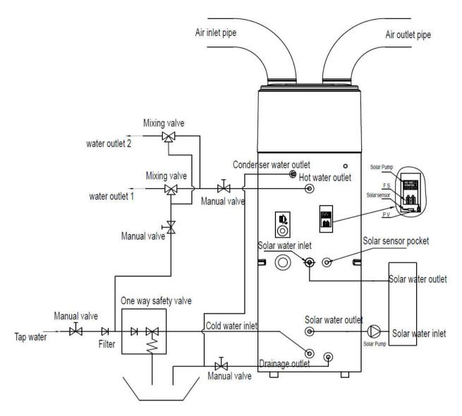
Note: 200S and 300S models have solar heat exchange coil.
