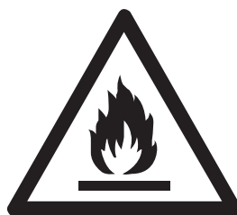
Caution: Risk of fire
