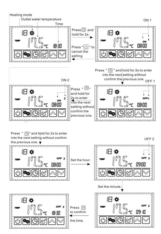
Example: Running period 1: 8:00~10:00; Running period 2: 16:30~22:00. ON 1 Outlet water temperature Current time Press " and hold for 2s Confirm the time after setting. OFF 1 ON 2 Confirm the time after setting. Confirm the time after setting. OFF 2
