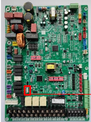
Main control PCB
