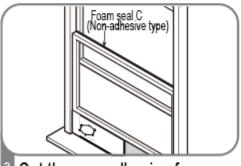
Cut the non-adhesive foam seal C strip to match the width of the window. Insert the seal between the glass and the window frame to prevent air and insects from getting into the room.
