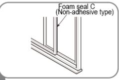
Cut the non-adhesive foam seal C strip to match the window height. Insert the foam seal between the glass and the window frame to prevent air and insects from getting into the room.
