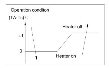
7.7.2.1. When TA < TS, the indoor fan operates firstly, and then the heater operates after 4 seconds.
