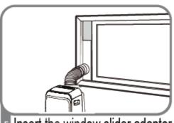
5 Insert the window slider adaptor into the hole of the window slider.
