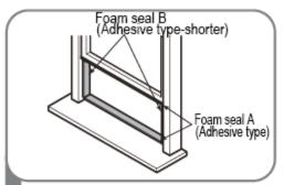
Cut the adhesive foam seal A and B strips to the proper lengths, and attach them to the window sash and frame as shown.
