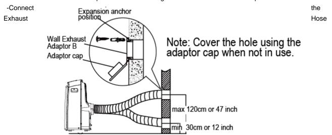
Assembly(with Wall Exhaust Adaptor A) to the Wall Exhaust Adaptor B.
